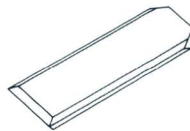
Inter-Contact Keying Plug, Part No. 88113-1
